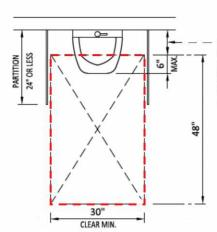
Space extending greater than 6 inches beyond the available knee clearance at 9 inches above the finished floor or ground surface shall not be considered to clearance.
